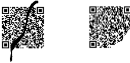
Figure 50. Damage and dirty resistant
